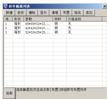
Figure 4.2.3 Diagonal-brace section list
